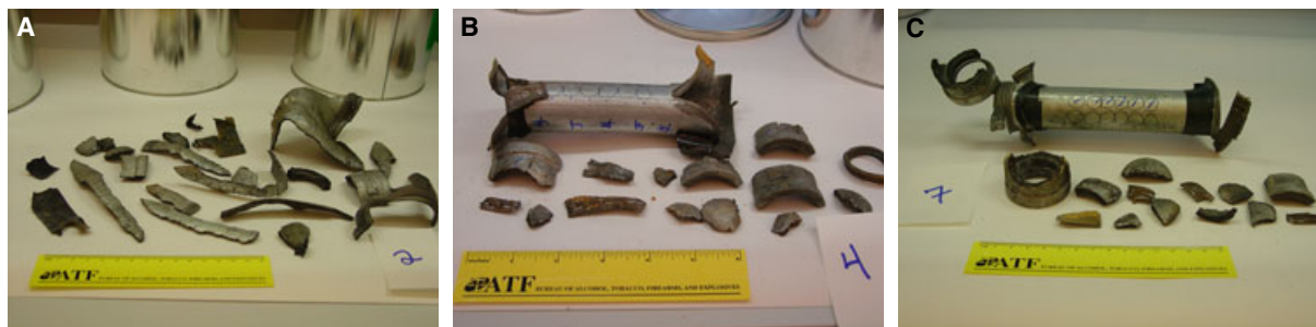
FIG. 1—Fragments collected from three of the devices post-blast. Different levels of fragmentation were observed depending on the brand of powder used in the device. The circles marking the areas where cell spots were deposited can be seen on some fragments. (A) Device #2, Go Ex Pinnacle, (B) Device #4, Jim Shockey's Gold, and (C) Device #7, Triple 7.
