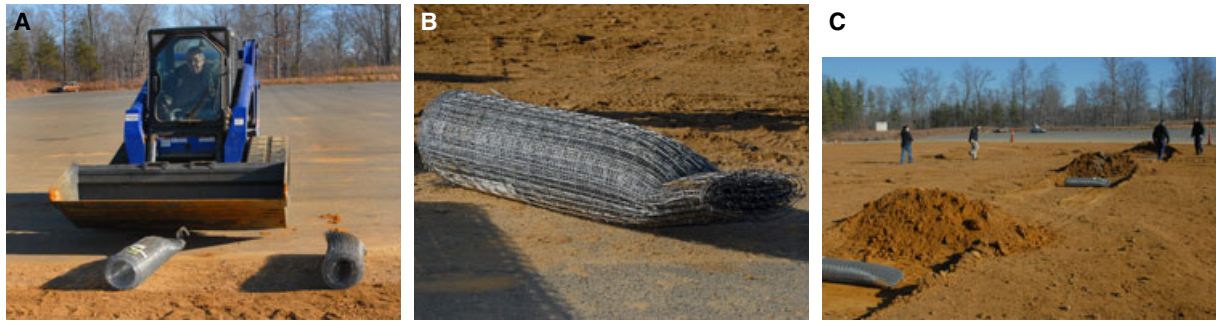
FIG. 2—Demonstration of how the devices were prepared to prevent cross-contamination of fragments and maximize the number of fragments collected. (A and B) The rolls of wire fencing were crimped on one end and (C) the rolls of wire fencing were placed in 2–3 foot deep trenches.
